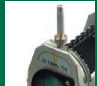
The tip may be flattened by 1/10 mm per point in a 90° position.
