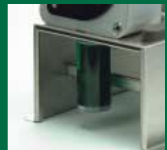
Sealed disposable container for toxic dust collection.
