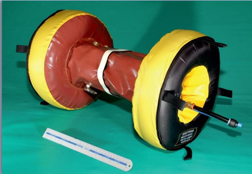
This Inflation Pipe Purge System makes an effective seal for purging pipework prior to welding. Once in position the bags inflate forming a tight seal inside the pipe. When inflated the pre-set purge valve will open, releasing inert gas into the weld area.
